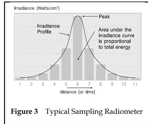
**Figure 3** Typical Sampling Radiometer
